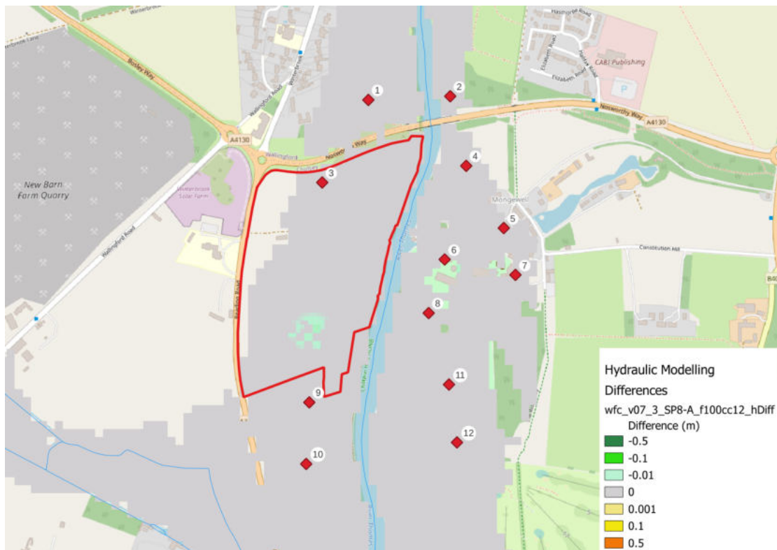
Figure 6.14: Flood Difference Mapping : Stage SP8 Flood Levels minus Baseline Flood Levels for a 1%AEP event with an allowance of 12% for climate change
